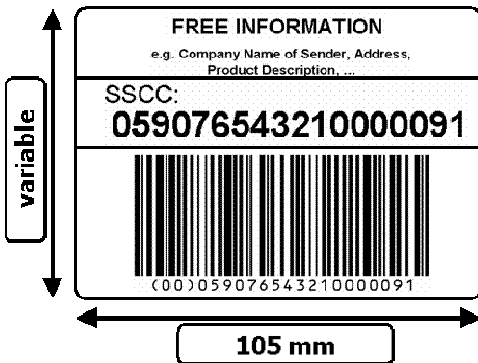
Figure 3. GS1 Logistic Label with SSCC only.
